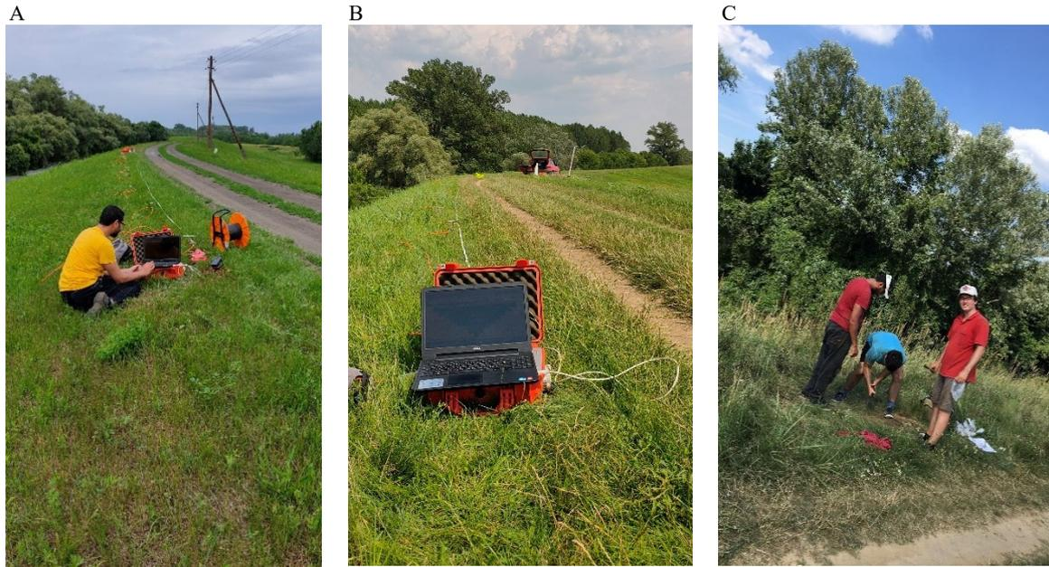
Fig. 2 Data acquisition by GEOTOM MK8E100 multi-electrode ERT system at 31.4 Lkm of Tisza levee (A), and 4 Lkm of Maros levee (B). Drilling boreholes by using an Eijkelkamp drilling system (C).
