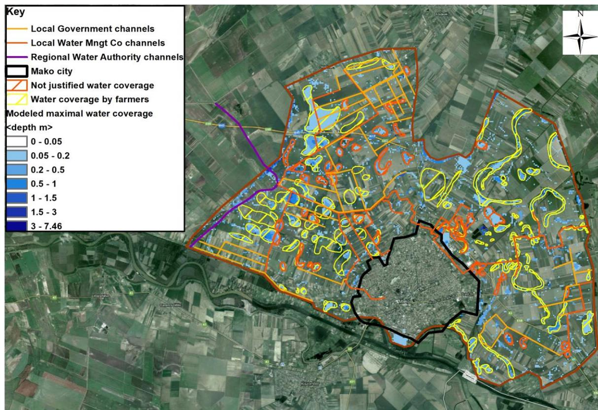
Fig. 3 Confirmed modelled maximal water coverage (1998-2000) by the local farmers in the Marosszög pilot area
